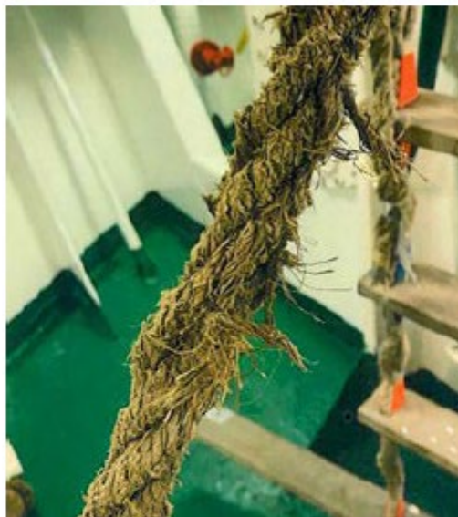
Photo 10: Frayed side rope.
