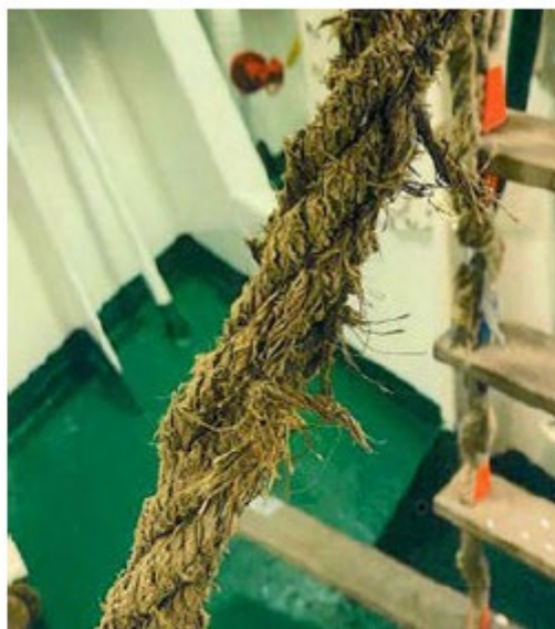
Photo 10: Frayed side rope.
