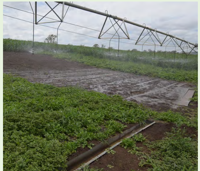
Image 2. Soil loss site with travelling irrigator and soil loss troughs. Note the runoff evident from the fallow treatment compared with no runoff from the cover crop treatment.
