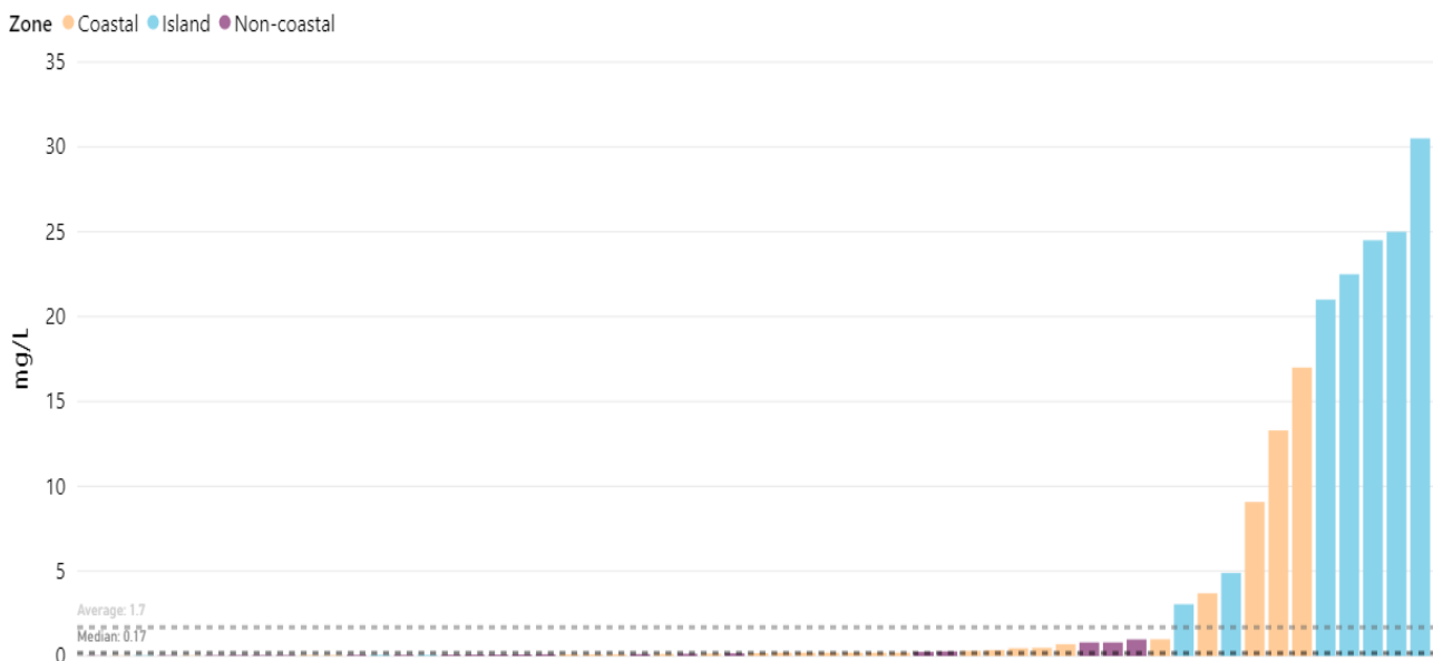
Figure 6-11. Selection of ammonia release concentrations for council STPs in the Reef catchment. Values are the median of all release monitoring data collected for that facility from 2017 and 2018. The dotted lines show the middle and average TN concentration value of all facilities (0.17 mg/L and 1.7 mg/L, respectively)
