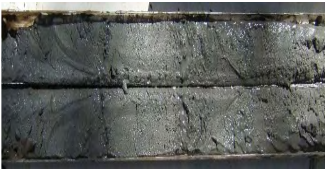
Figure 10. Dark grey fine sandy PASS layer at 6m depth, S P 5+ map unit.
