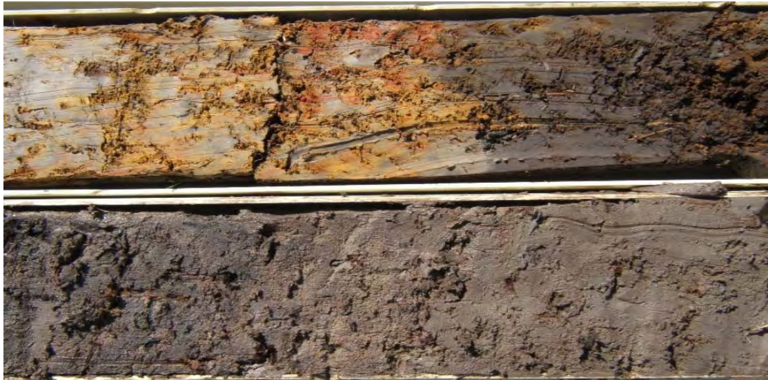
Figure 5. AASS layer with yellow jarosite over grey PASS layer, A0S1 map unit.
