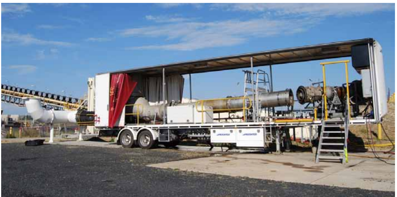
Figure 9: QMRS trailer mounted GAG unit
