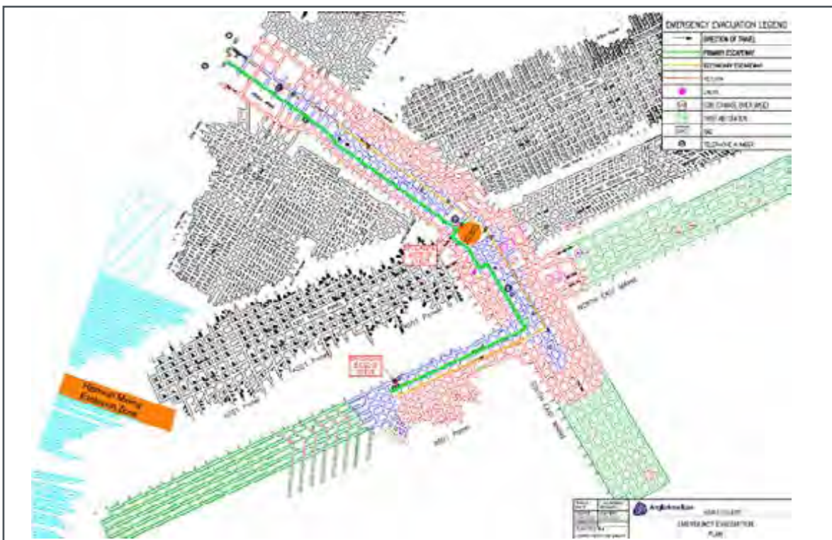
Plan of Aquila Mine workings (Courtesy Anglo American Metallurgical Coal)
