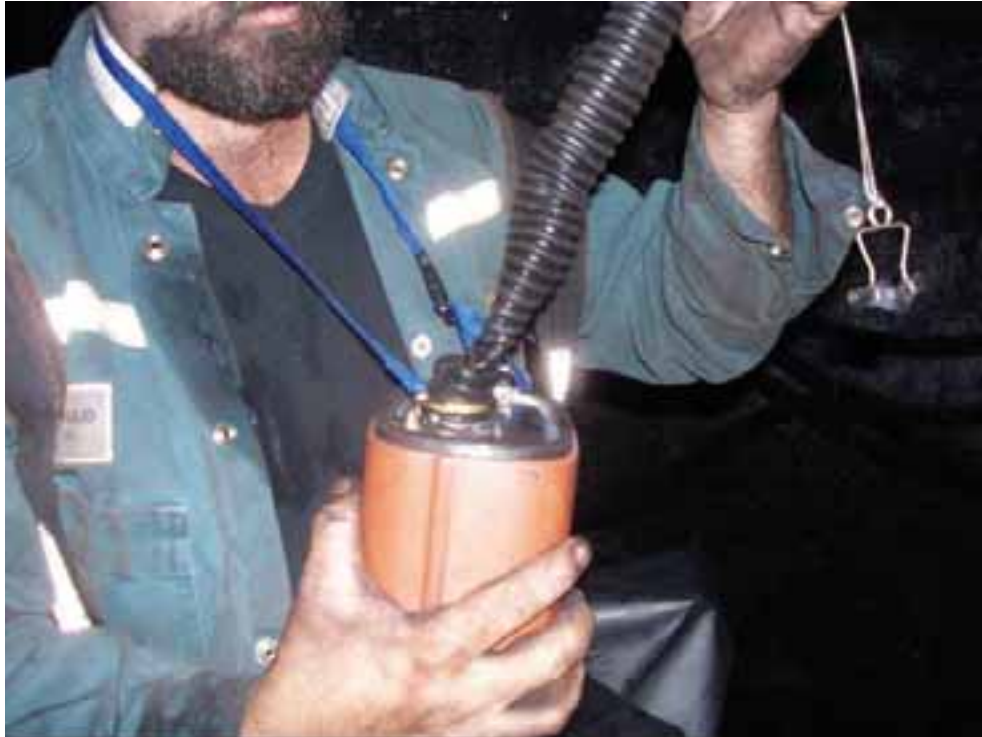
Figure 5: Collapsed SCSR hose
