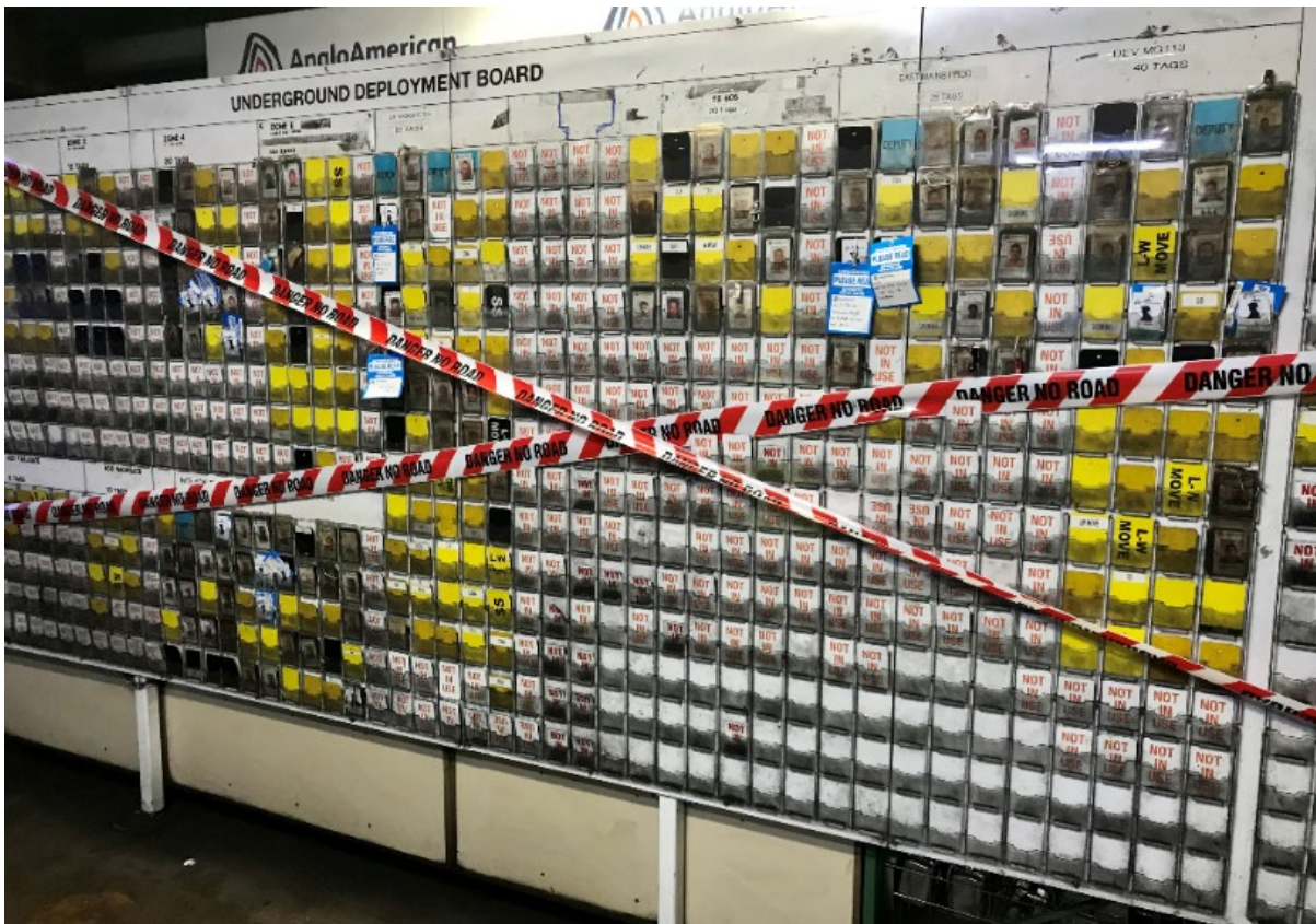
Figure 7 Surface tag board (note the danger tape covers some of the tags)
