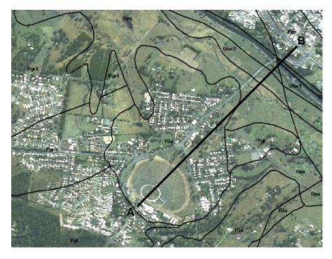
**Plate 42 Cross-section (A-B) of the Mary River, Gympie** (see Figure 9) This involves elevated paleo-alluvial deposits (TQa) of Land Zone 5 elevated above the recent alluvium (Qha, Qpa) of Land Zone 3. Pgs rock represents Land Zone 11 (Google Earth)
