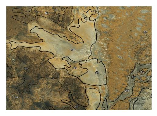
Plate 25 Wind-blown sand plains (S2) of Land Zone 5 overlie paleo-alluvial clay plains (F6) of Land Zone 4 south of Winton.
