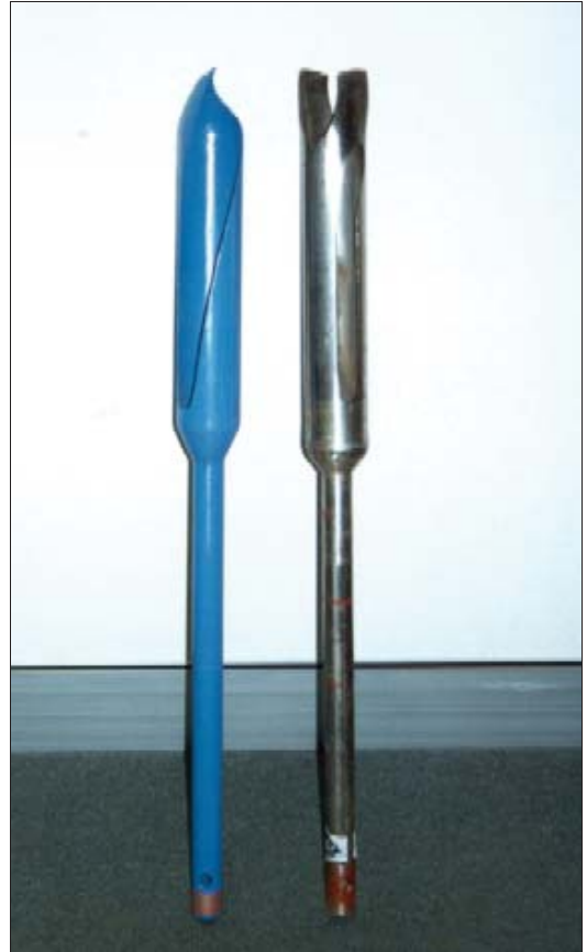
Plate 2. Dormer soil and Dormer sand augers
