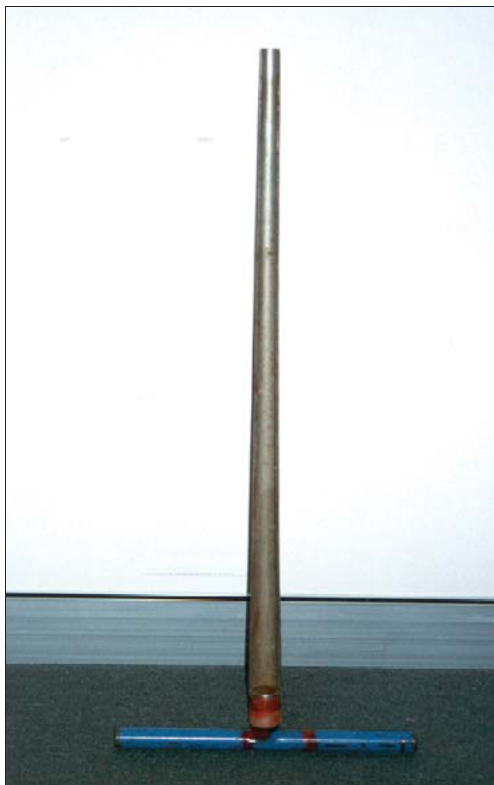
Plate 3. Dormer tapered gouge auger
