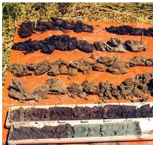
Photograph 2: Soil profile laid out on a tarpaulin in 1 m segments: note the gley, Pleistocene, heavy clay basement core sample in the PVC tray at the knife tip
