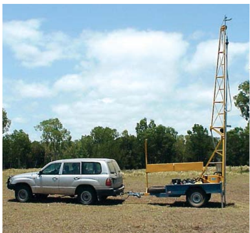
Photograph 1: Vacuum-vibro coring rig used for deep sampling of ASS
