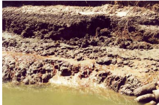
Photograph 28: Iron staining on the gley, Pleistocene clay basement from oxidation of the overlying PASS in the McEwens Beach prawn farm intake channel
