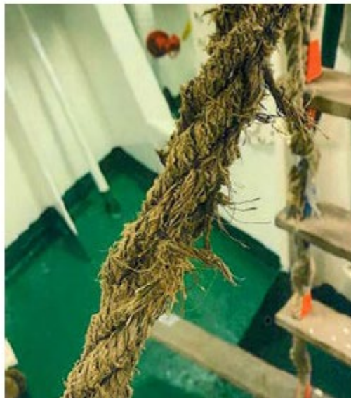
Photo 10: Frayed side rope.
