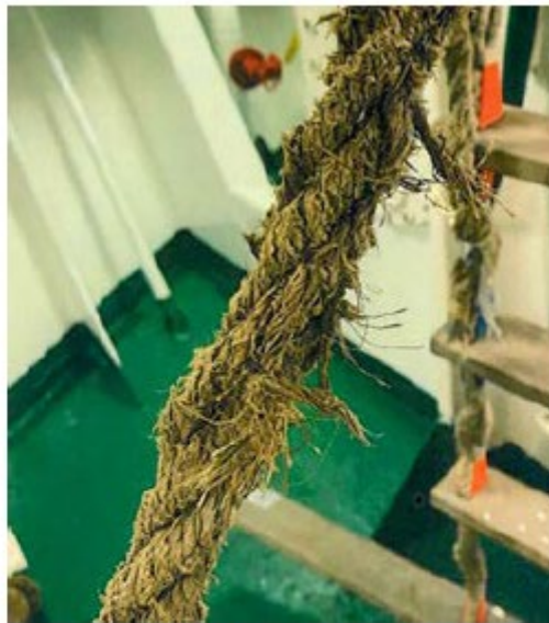
Photo 10: Frayed side rope.
