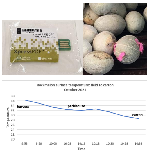
Image 5: USB temperature logger (top left), USB-logger strapped to a melon (top right) and graph generated by measuring temperature from the field to packing (bottom).
