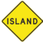
Raised area on road
