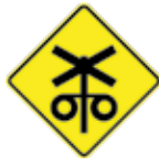
Railway level crossing – flashing signal ahead
