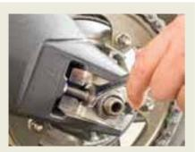
**Chain** — ensure the chain has the correct tension, not too tight or too loose, and is appropriately lubricated.
