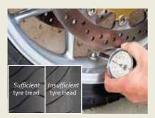
Tyres — ensure the tyres are in good condition and are wearing evenly. Check that they have a tread depth of at least 1.5mm across the tread surface, and are inflated in line with the manufacturer's recommendations.
