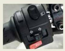
**Lights** — ensure all lights (headlights, tail lights, brake lights) and indicators are clean and operational.
