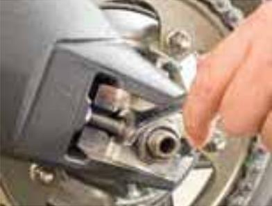
**Chain** — ensure the chain has the correct tension, not too tight or too loose, and is appropriately lubricated.
