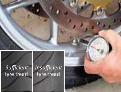
**Tyres** — ensure the tyres are in good condition and are wearing evenly. Check that they have a tread depth of at least 1.5mm across the tread surface, and are inflated in line with the manufacturer's recommendations.
