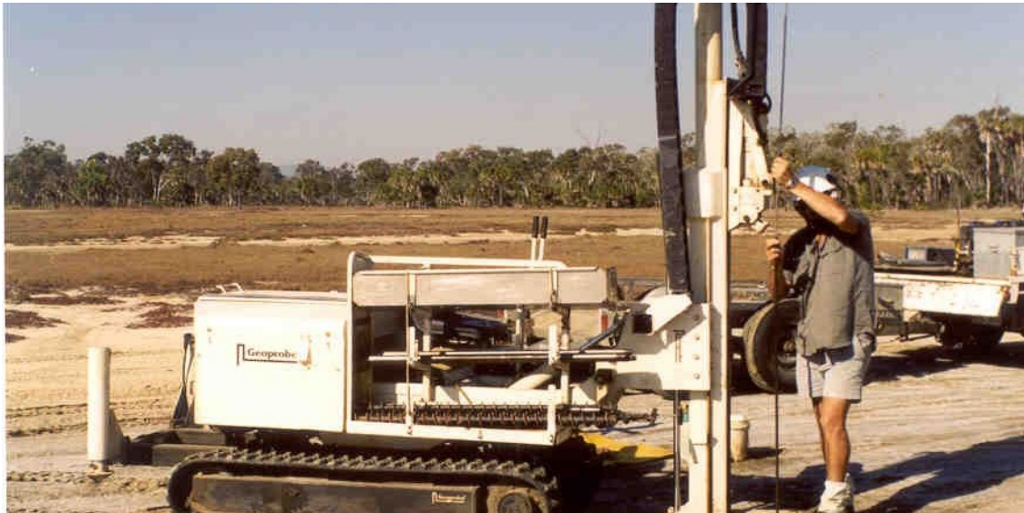
Figure 3. Geoprobe core sampling, chenier plain, Keppel Sands.
