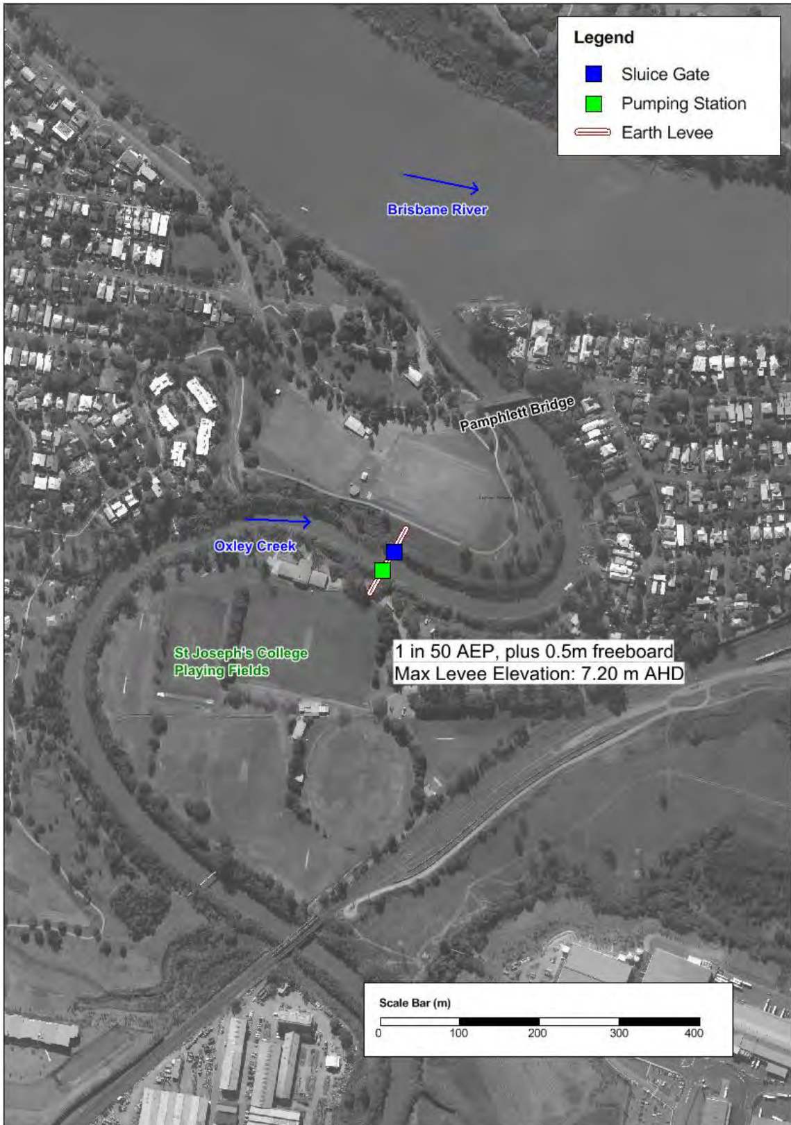
Figure 8-22 Location of Oxley Creek levee and sluice gates
