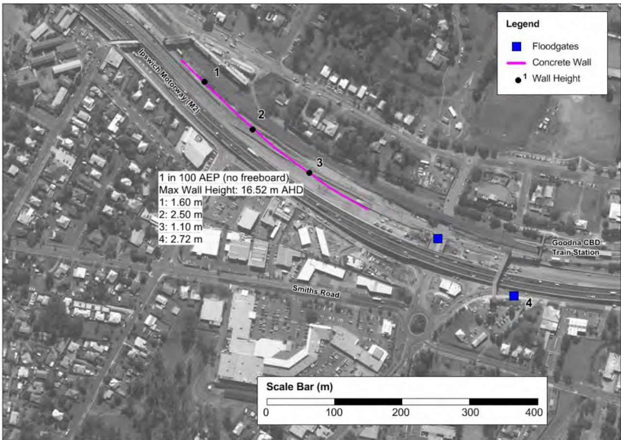
Figure 8-14 Location of Goodna CBD wall and floodgates
