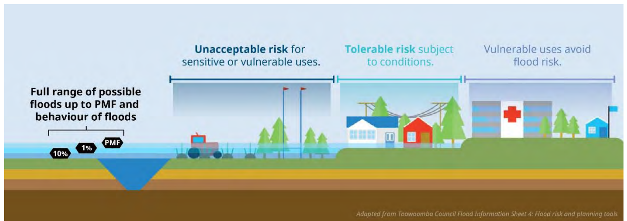
Figure 9-2 Concept of risk-based planning (adapted from Toowoomba Regional Council Flood Information Sheet 4 – Flood risk and planning tools)
