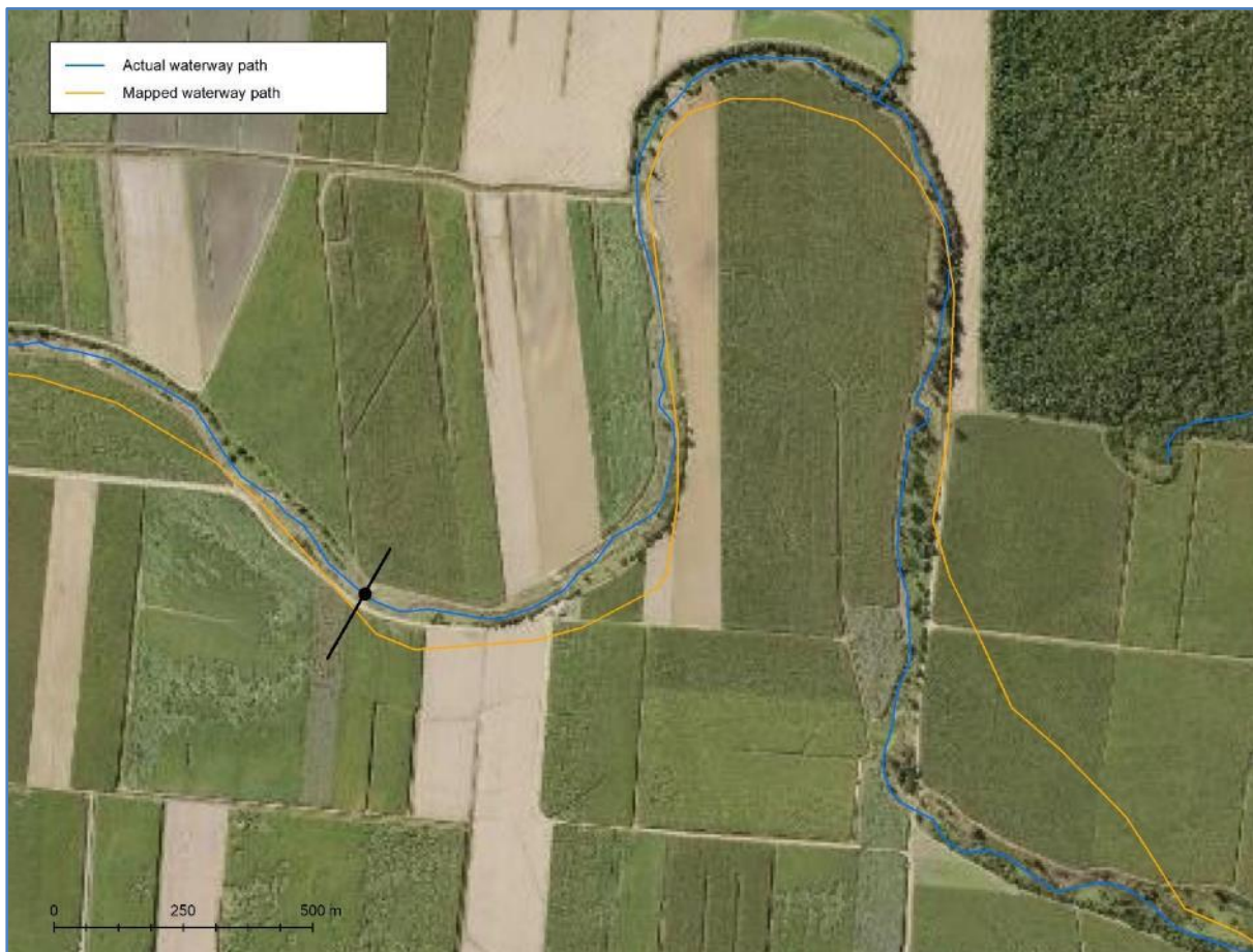
Figure 3: Example of a misalignment of a mapped waterway with the on-ground waterway
