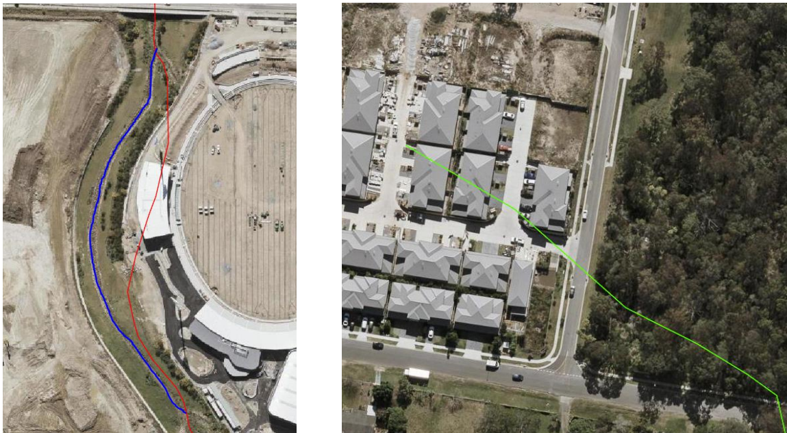
Figure 4: Examples of the waterway mapping no longer reflecting the on-ground features – (left) a red waterway that has been diverted around a sporting complex and (right) the upper end of a green waterway that has been filled and no longer exists on ground
