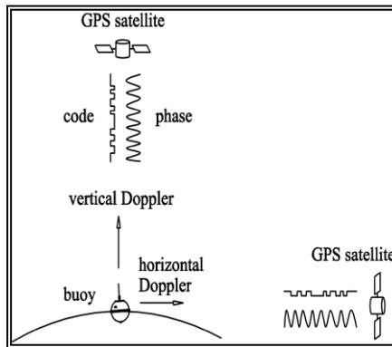
**Figure 2 The GPS wave measurement principle (Datawell, 2010)**
