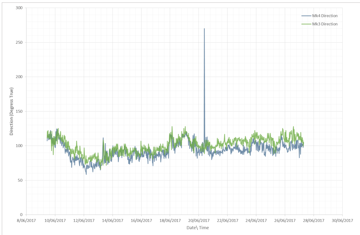
Figure 11 A 20-day comparison of Tweed Wave Buoy data. (Mk4 direction is in degrees magnetic and Mk3 is in degrees true)
