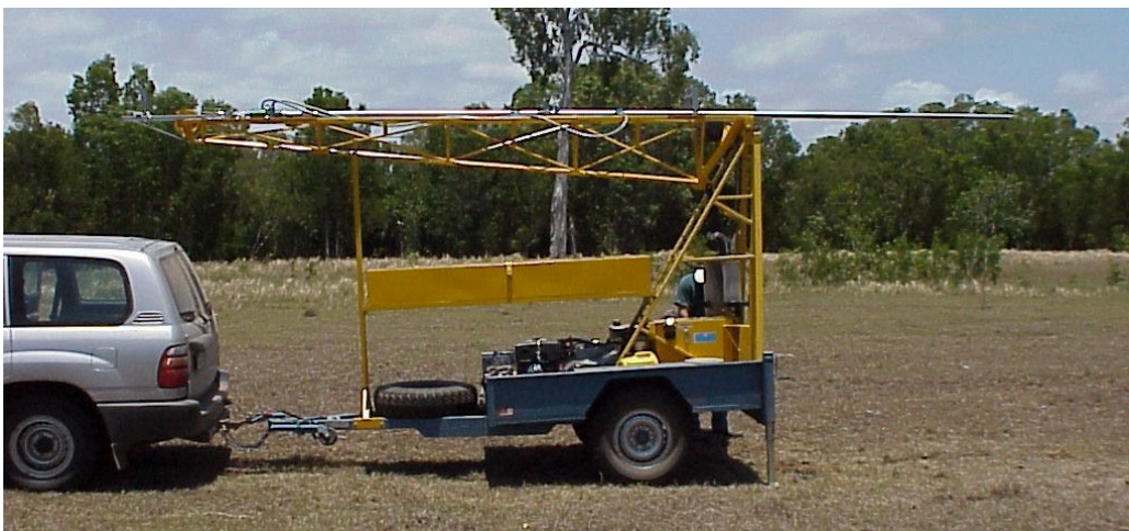
Photograph 3. Trailer mounted vibro-coring soil rig used for sampling wet sediments
