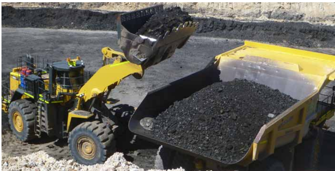
Komatsu WA900 loading a Komatsu 15500 rear dump truck Photo: DNRM
