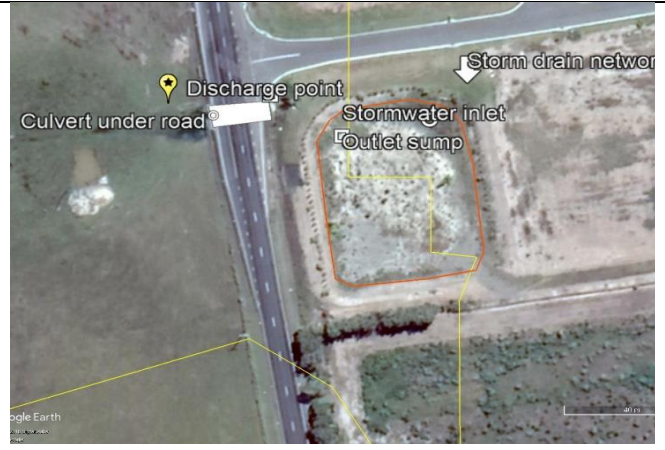
Figure 13 Stormwater inflow to wetland from housing estate bio-retention pond – aerial view (C. Johns, 2018). Bio-retention pond outlined in red. Wetland boundary in yellow. Yellow map marker shows photo point for previous image (left). Water diverted to bio-retention pond from estate storm drain network leaves via an outlet sump that discharges downslope, running into the wetland through a box culvert under the road.
