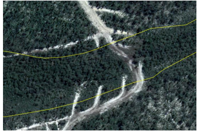
Figure 15 Aerial view of road with drains diverting water to wetland. Wetland boundary in yellow. Roadway runs through wetland north-south with 8 to 9 drains branching off.
