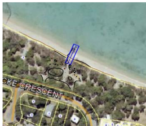
Figure 1: Proposed concept design for Dingo Beach boat ramp short extension
