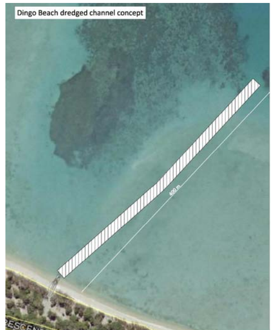
Figure 2: Proposed concept design for Dingo Beach dredged channel
