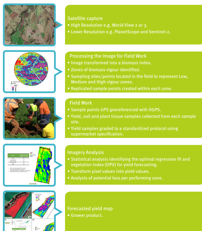
Figure 2. A schematic of the process from satellite capture to creating the forecasted yield maps for the grower.
