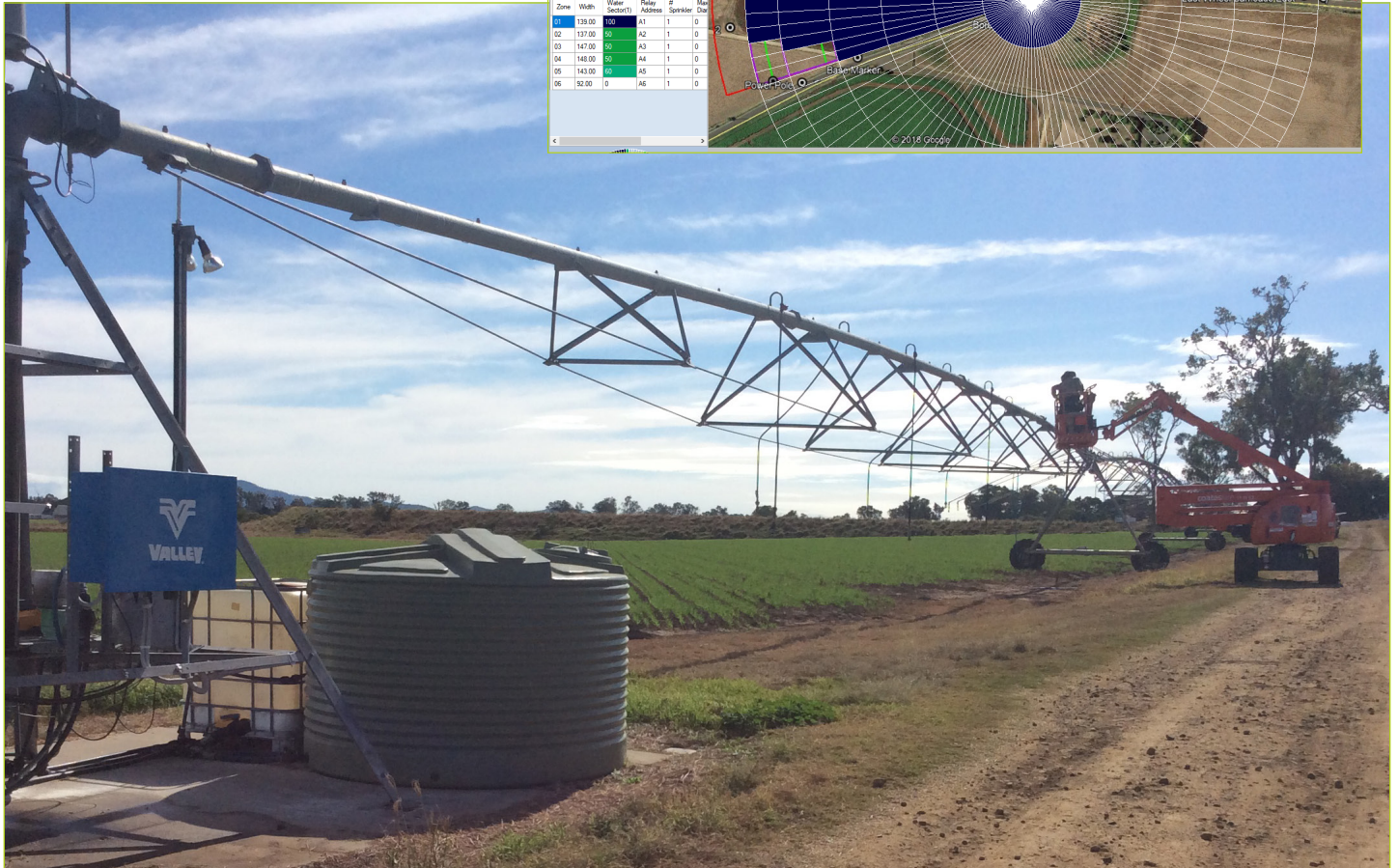
Figure 5. Retrofitting of VRI capability to a centre pivot irrigator for vegetable production.
