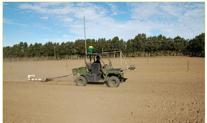
Figure 2. An EM38 Sensor towed behind a quad bike to assess soil variability in a fallow field. Source: DAF QLD (2014)
