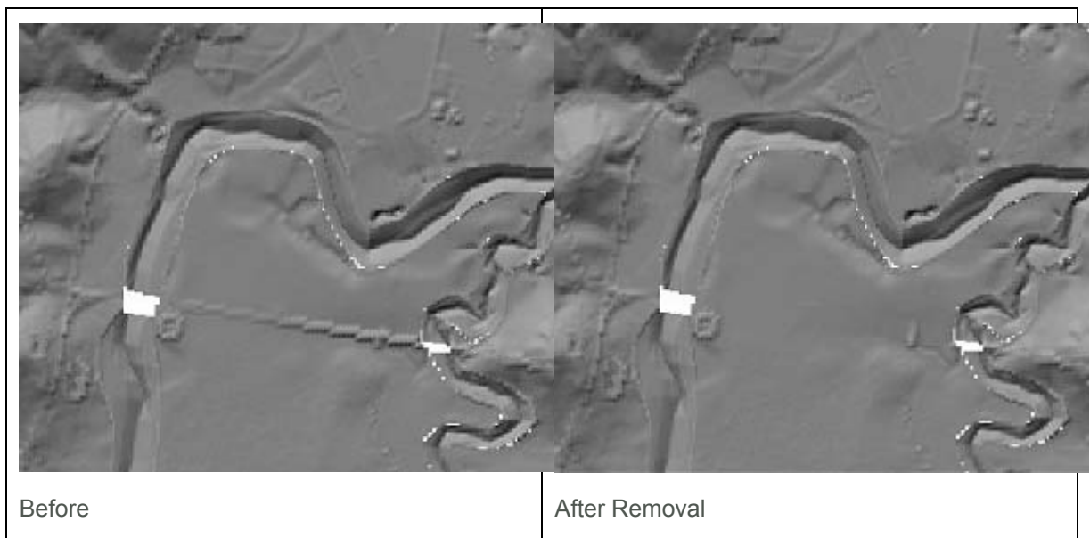
Figure 2-1 Removal of Cunningham Highway Raised Section for 1974 Topography
