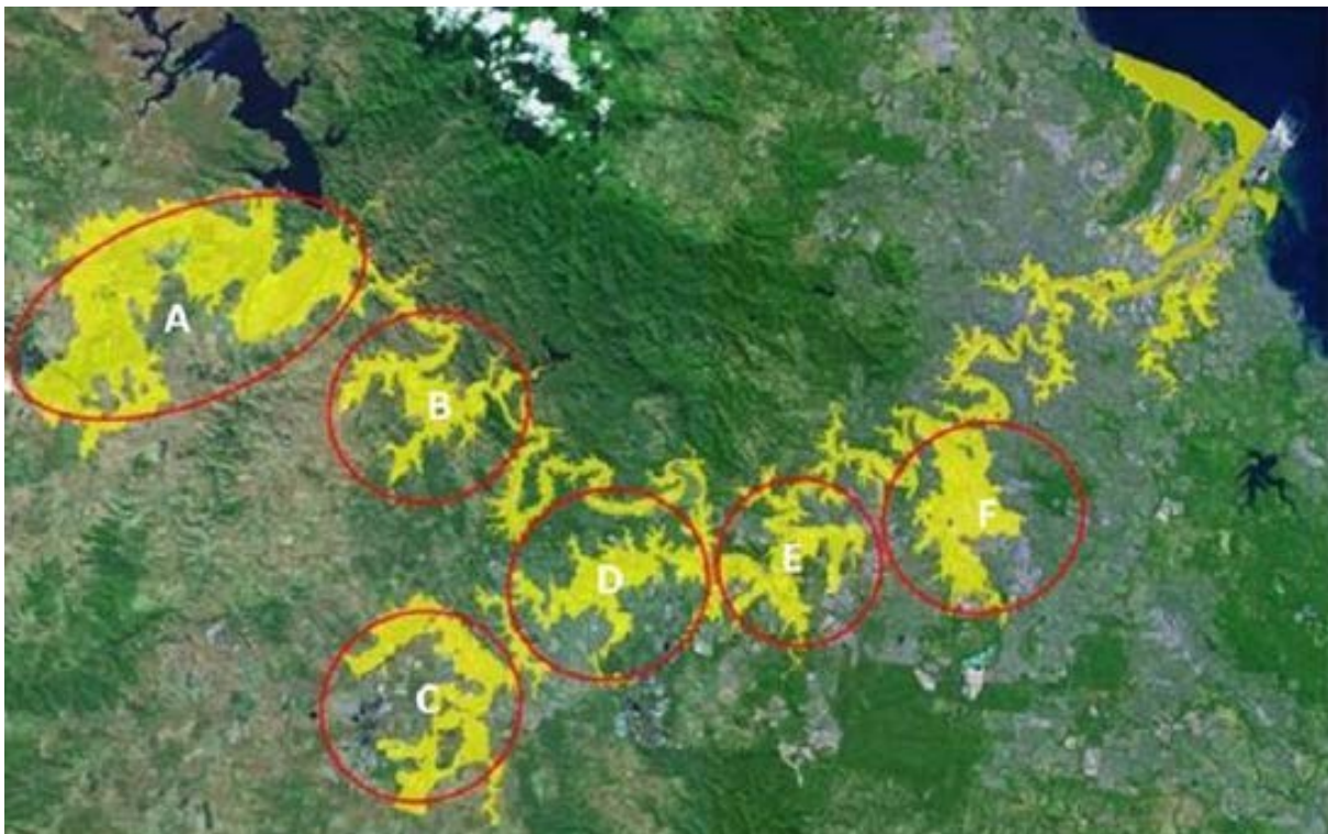
Figure 3-9 Seqwater Figure 7-95: Conceptual flood storages – Lower Brisbane River
