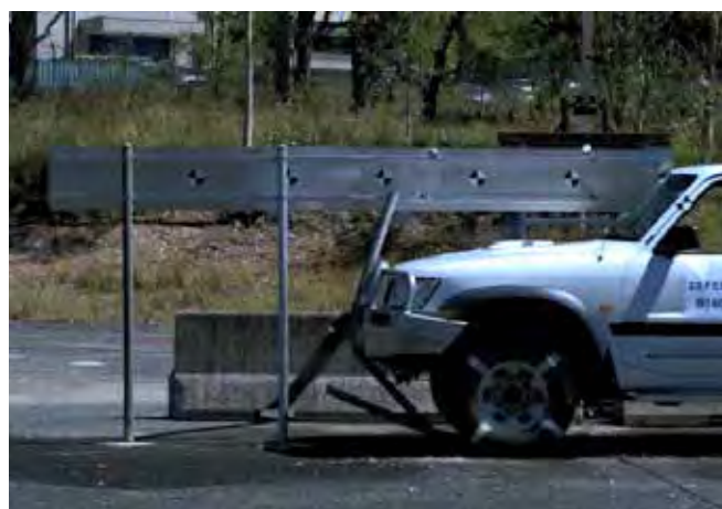
Test undertaken without sign spearing technology.
