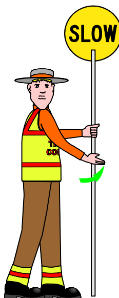
Figure 4.6.3 TO DIRECT TRAFFIC TO GO
