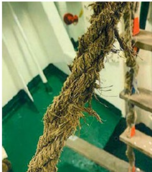
Photo 10: Frayed side rope.
