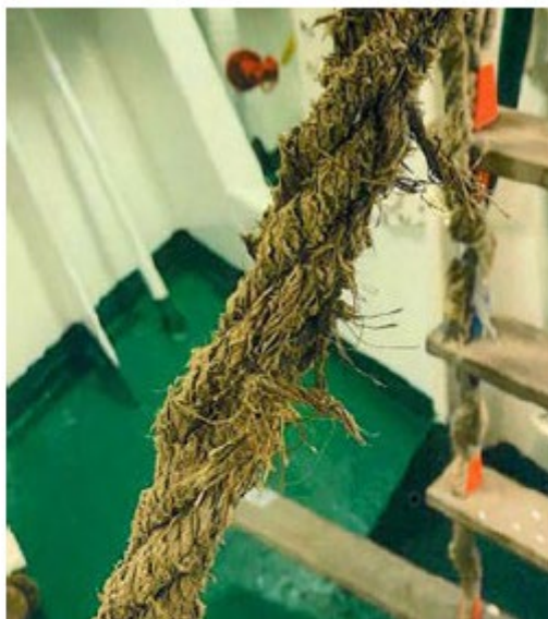
Photo 10: Frayed side rope.
