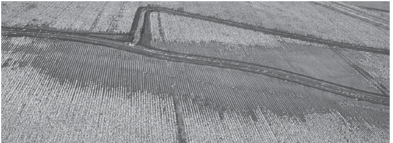
Figure 9. Soil salinity effects on irrigated cotton due to evaporation from shallow groundwater in the Emerald Irrigation Area, Queensland. The problem was reclaimed with the installation of shallow drainage.
