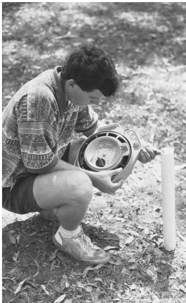
Figure 45. Measuring the groundwater depth and groundwater electrical conductivity simultaneously in a piezometer.
