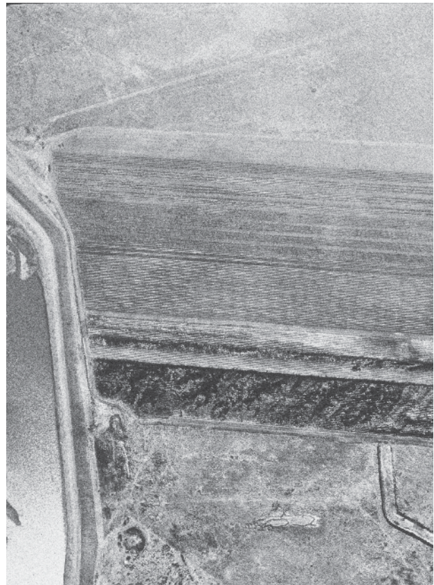
Figure 71. Linear pattern of salting as a result of geologic dykes below a leaking farm dam in the Lower Burdekin, Queensland.
