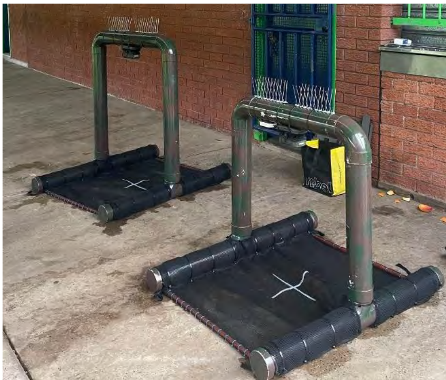
Figure 37 Pontoons for detecting juvenile REST assembled and ready for field testing
