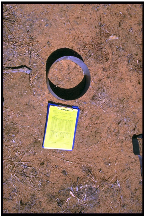
Photo 9. Infiltration on bare topsoil
