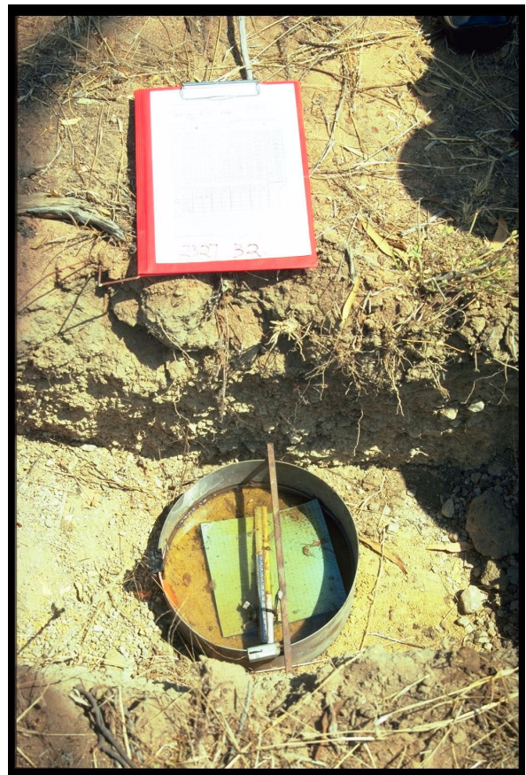
Photo 10. Infiltration on top of B horizon
