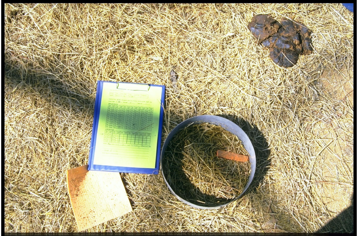
Photo 8. Infiltration on surface soil under grass cover
