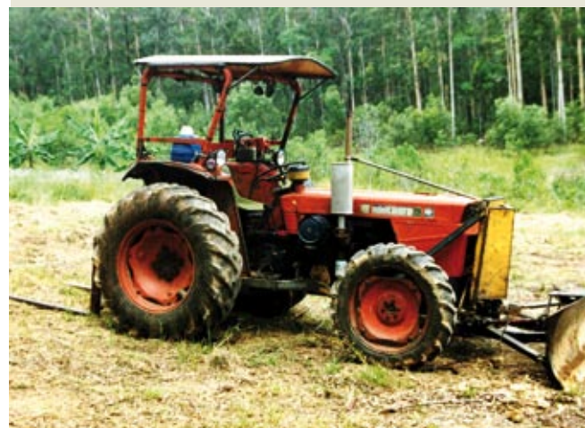
Figure 1.3 The tractor used for the harvest was a 60 hp 4WD with blade and rear forks.
