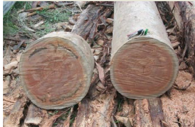
Figure 3.3 Butting the log to remove defect associated with the stump, which in this case was most likely an old fire scar.
