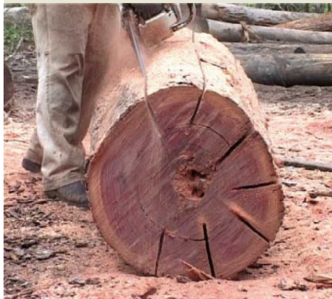
Figure 4.11 Splitting posts from a bloodwood log. Posts are wedged apart from the ring, which pops as the cuts are made.
