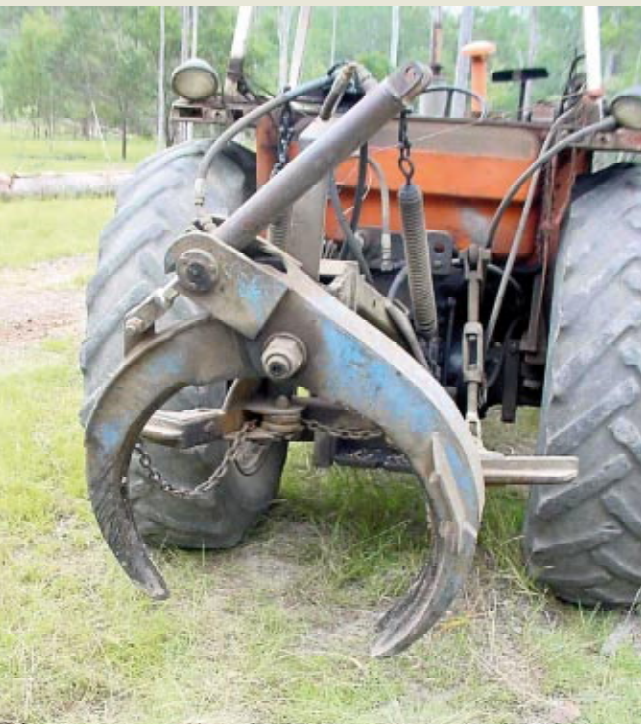
Figure 3.4 A tractor and hydraulic grapple used for snigging.
