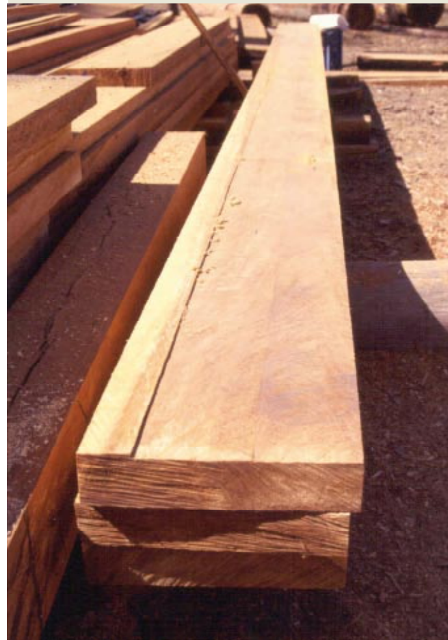
Figure 3.6 A variable-depth sawn groove was often left on boards wider than 200 mm.
