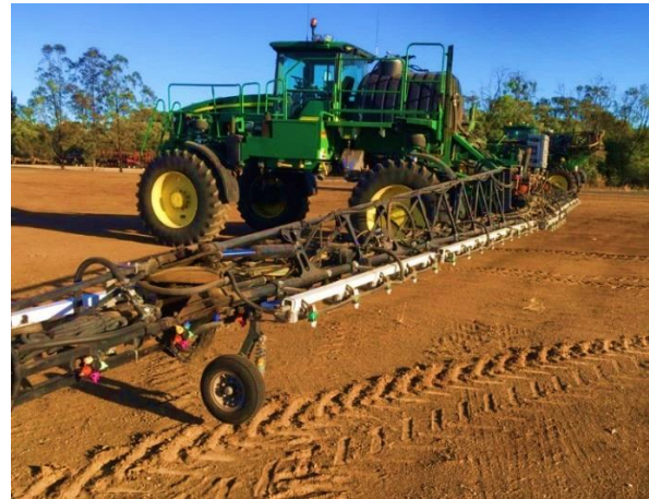
Figure 1: The Wagner's 24m John Deere 4730 with Weedseeker 2 cameras retrofitted. Photo: Mark Wagner.
