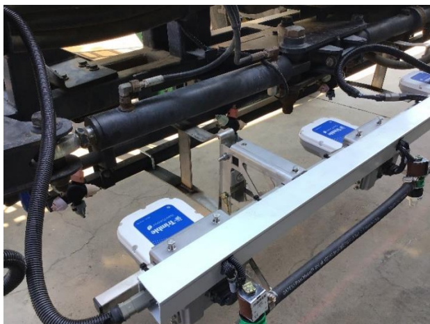
Figure 2: Weedseeker 2 cameras fitted with quick release stainless steel brackets. Photo: AgSpray.
