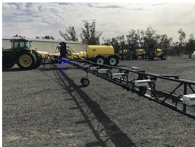
Figure 2: Extended 36m Hayes trailing boom. Photo: Hayes.
