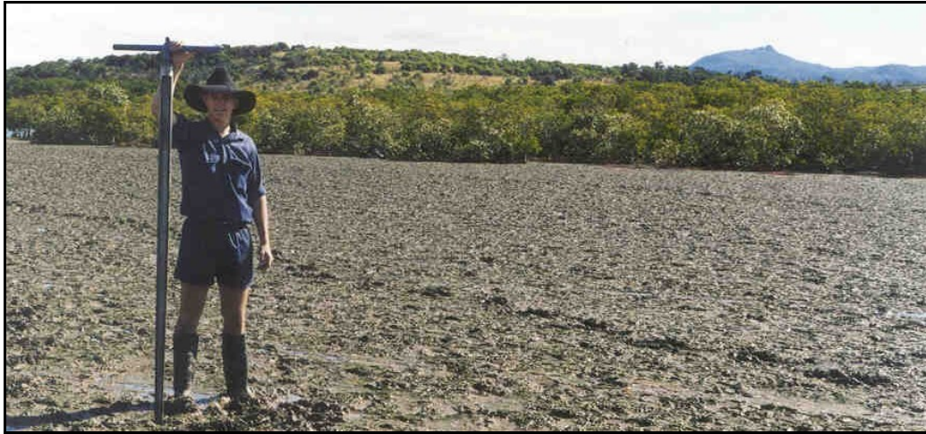
Photograph 2. Gouge auger, 1.8 m long, used for hand sampling in mangrove forests
