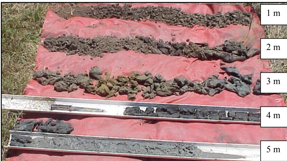
Photograph 13. Soil of the Proserpine River floodplain with PASS (dark grey sediment at end of third row of soil) beginning at 2.8 m, S 3 map unit
