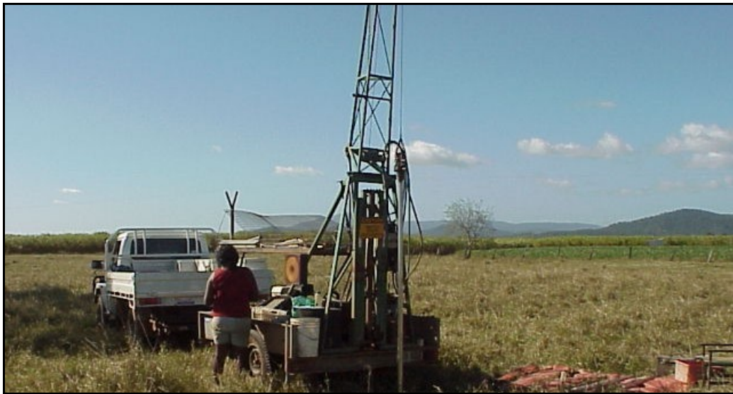
Photograph 3. Trailer mounted vibro-coring soil rig used for sampling wet sediments
