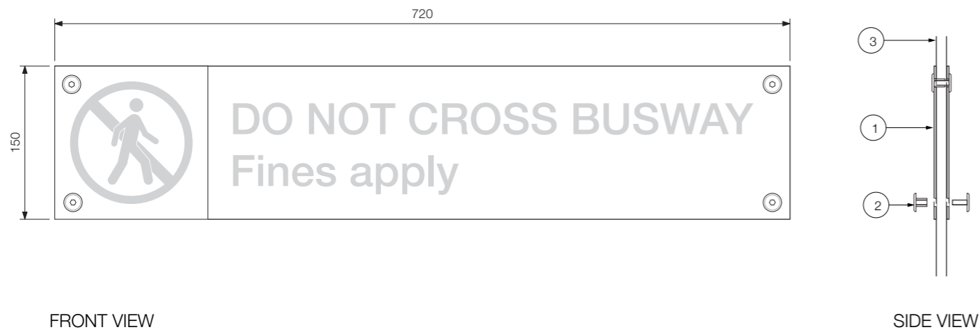
Construction Detail – Mesh fence mounted Scale 1:5
