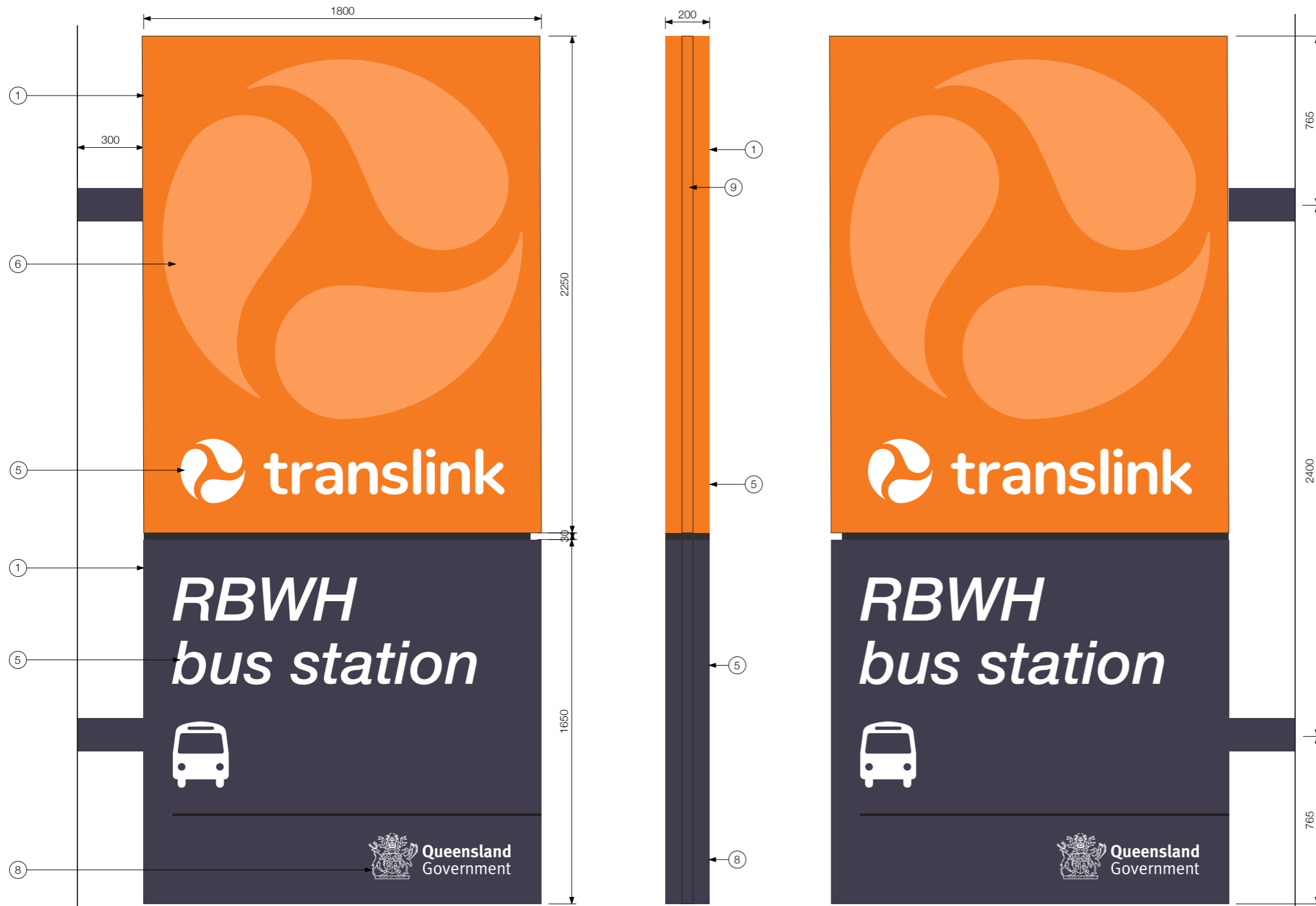
Sign Elevations Scale 1:20
