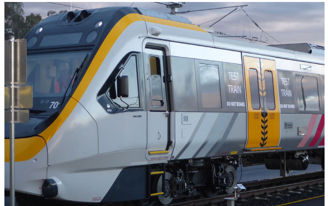
The first New Generation Rollingstock train being readied for on-track testing.
