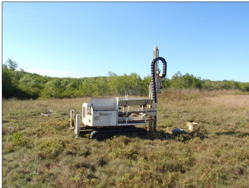
Plate 1. Geoprobe model 54DT track-mounted coring machine
