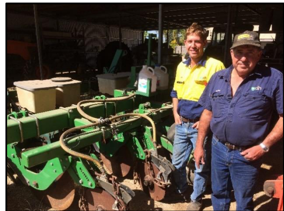
Figure 5.1: Sam and Gerry Deguara alongside their modified subsurface Dunder applicator
