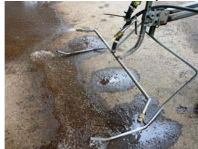
The spray bar showing centre air induction nozzle for glyphosate
