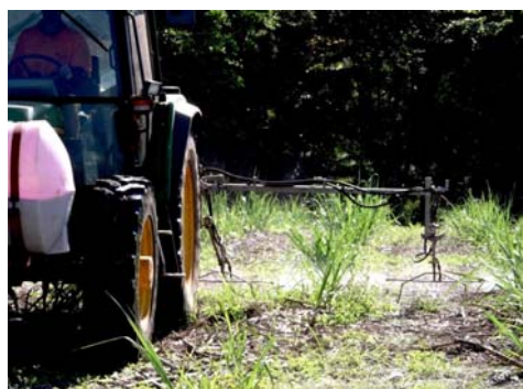
Dual herbicide sprayer operating. Note front glyphosate tank. Pink colouring is UV tracer used in calibrating the sprayer.
